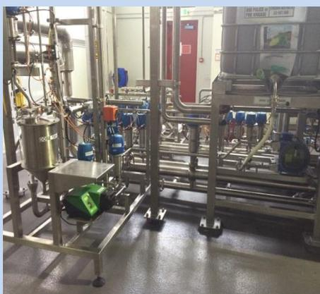
For the dosage options a wide range of flexibility is available to the brewer. The system has the capability to dose from day pots (10Lts), bulki's (IBCs) and a mixing tank (1300 Litres). The dosage rates available to create the new beer styles range from 0.010 g/litre to 15 g/litre depending on the dosing requirement.
